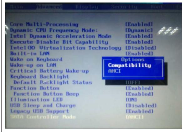
4. After test, remember to set SATA Controller mode back to "AHCI".
